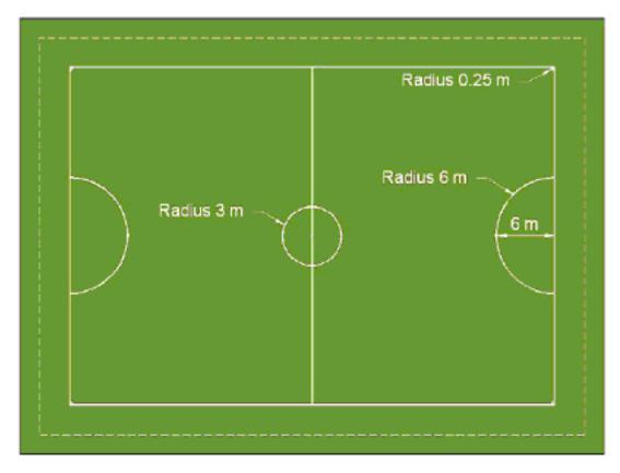
The two long (solid) boundaries are the touchlines; the two shorter solid lines are the goal lines. The dotted lines show the run-offs.
